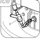
Check the spark plug gap with a feeler gauge and set at 0.7 - 0.8mm.
